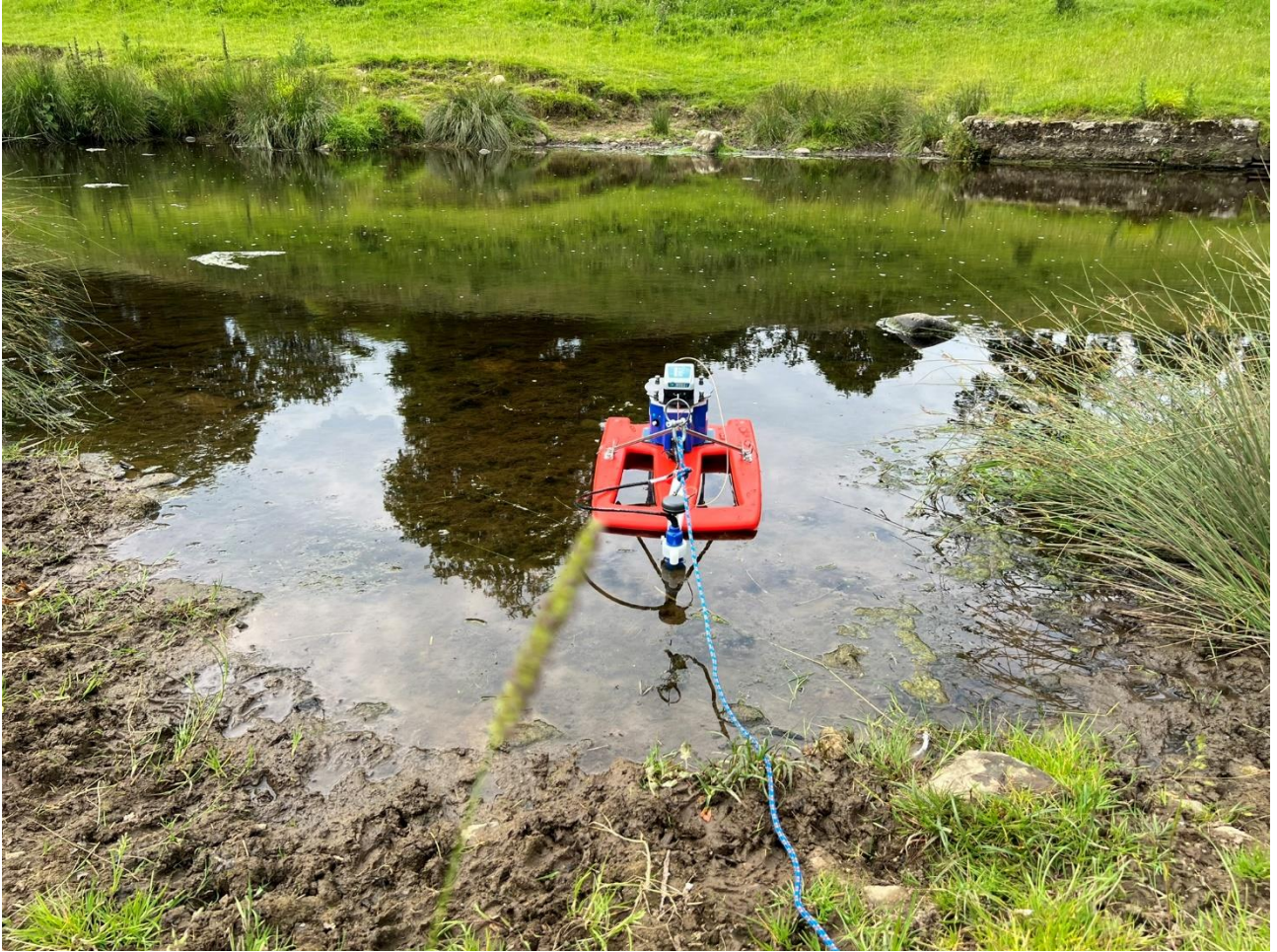
ADCP in river to record the depth and flow velocity.
