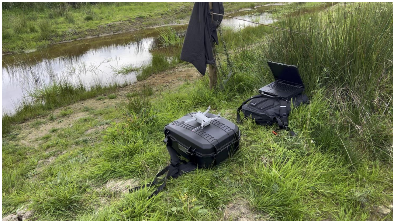
Drone to record area of NBS intervention to calculate storage duration.
