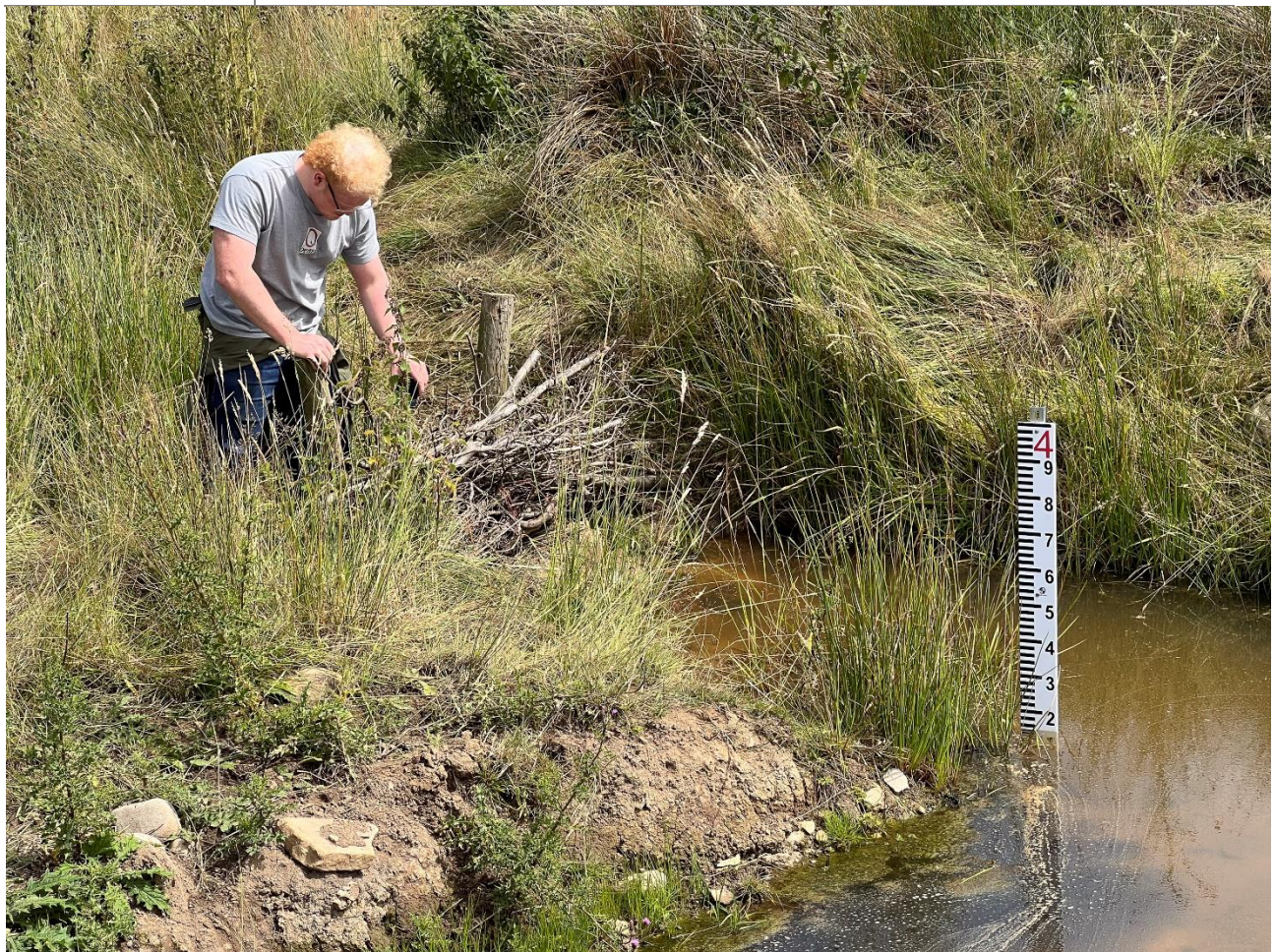
Picture of person next to leaky woody dam with a level board in front of the dam to show the height of the water retained.
