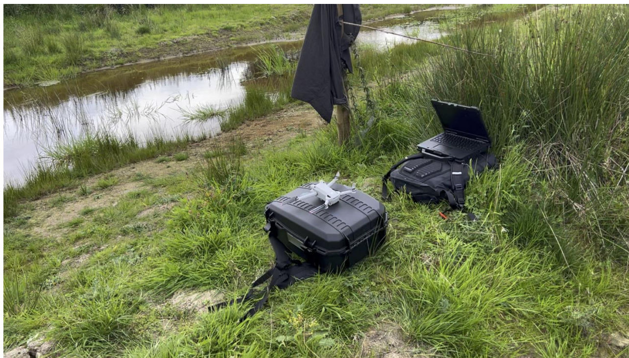
Drone to record area of NBS intervention to calculate area, roughness and evidence of channelised flow.
