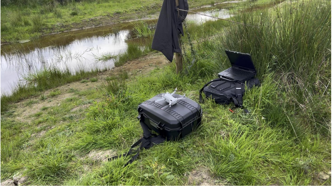
Drone to record area of NBS intervention to calculate area, roughness and evidence of channelised flow.
