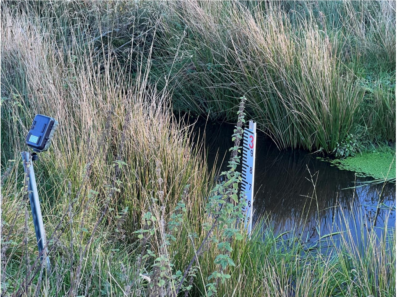
Level board to show depth of water and trail camera to take timelapse pictures of the board to record changes.
