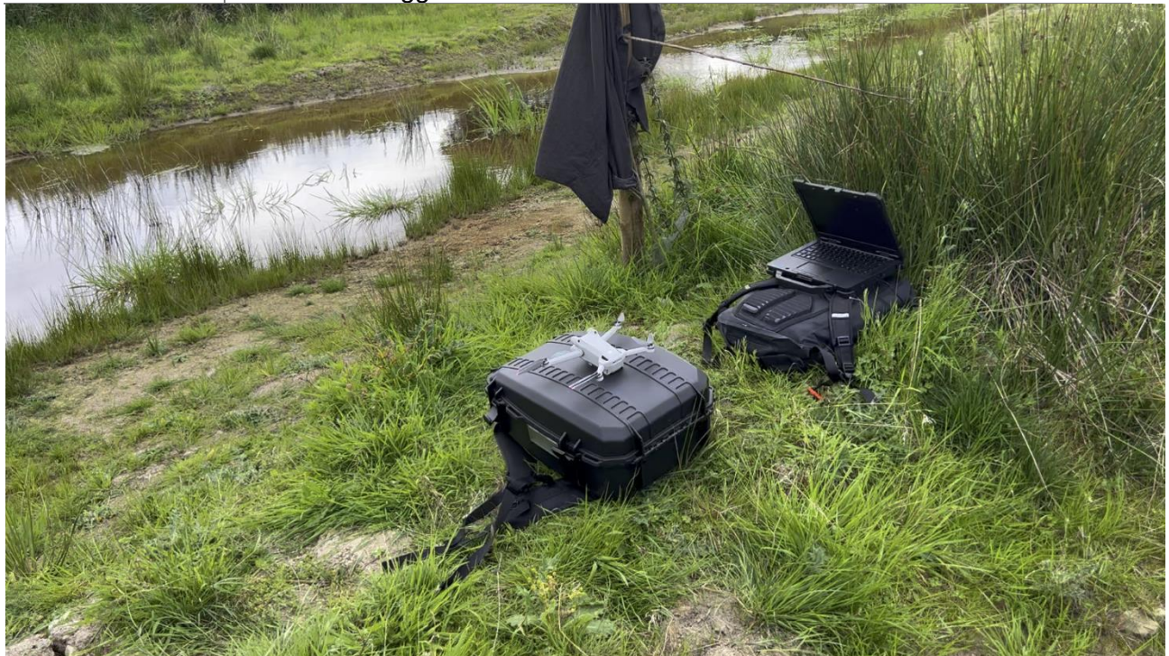
Drone to record area of NBS intervention to record evidence of channelised flow.
