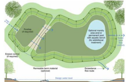
Figure 22.2: Plan and elevation of vegetated detention basin
